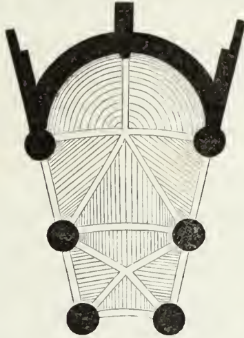
No. 1.—Plan of the vault of one compartment of the double aisles, according to Wilars de Honecort.
